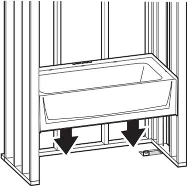
Install drain assembly per manufacturer's instructions. Place base into framing pocket.
