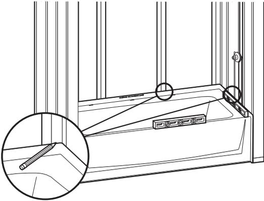
Level and mark all sides. Front apron should be firmly on the floor.
