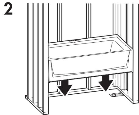
Check dimensions. **NOTE:** If you're adding additional accessories such as a grab bar—additional framing may be needed for support.
