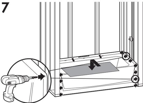
Pre-drill horizontal flanges along top of base section and fasten into each corresponding stud. Pre-drill both (vertical) side flanges and fasten to side studs 8" (200mm) on center. Place cardboard to protect finish.
