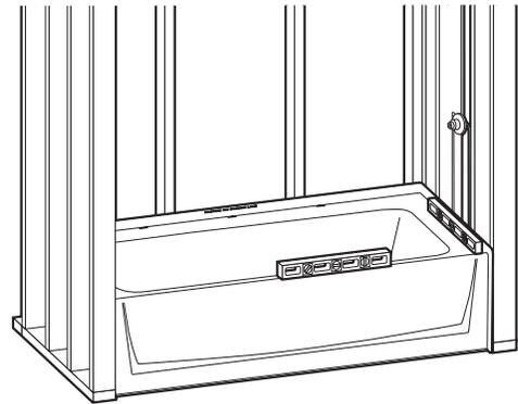
Level lengthwise and widthwise using 3 ft. (915mm) level by shimming if necessary. The unit must be set level.
